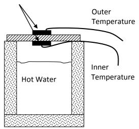
Observe the graph of temperature vs. time and wait until the two curves (the inner and outer
