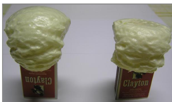
Prepared polyurethane foam, on the left PUR foam formed on the wet box.
