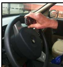
Controls mounted directly on the wheel
