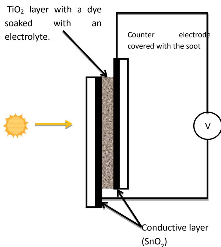
Figure 13. A diagram of the solar cell.
