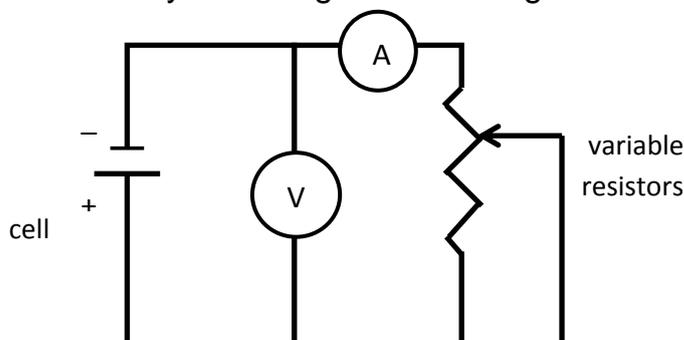
Figure 14 A diagram of a circuit for the measurement of the voltage-current characteristic.
