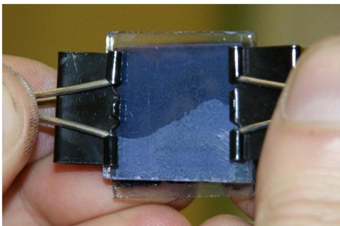
Figure 12. The plates combines with the paper clips after dropping an electrolyte.
