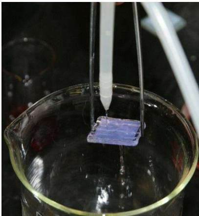
Figure 10. Rinsing the plate with methanol.
