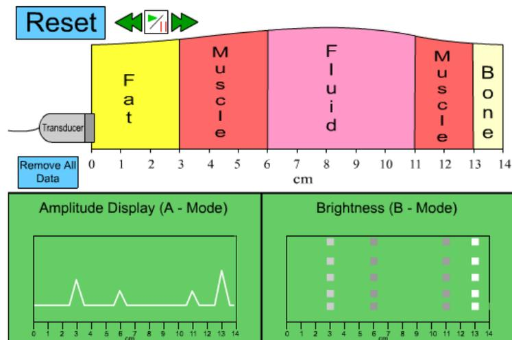
Then by using the simulation *Ultrasound Imaging with Object* <http://physics.doane.edu/hpp/Resources/Media/Flash/UltraSoundImagingwithObject2.html> students create a new scan. This time there is an extra object inside the body.
