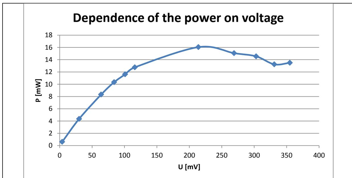
Figure 16. An exemplary dependence of the power on voltage for the working blueberry cell.
