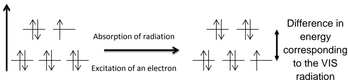
Figure 3. Diagram of d-type orbitals splitting and the electronic excitation for the octahedral coordination compounds.
