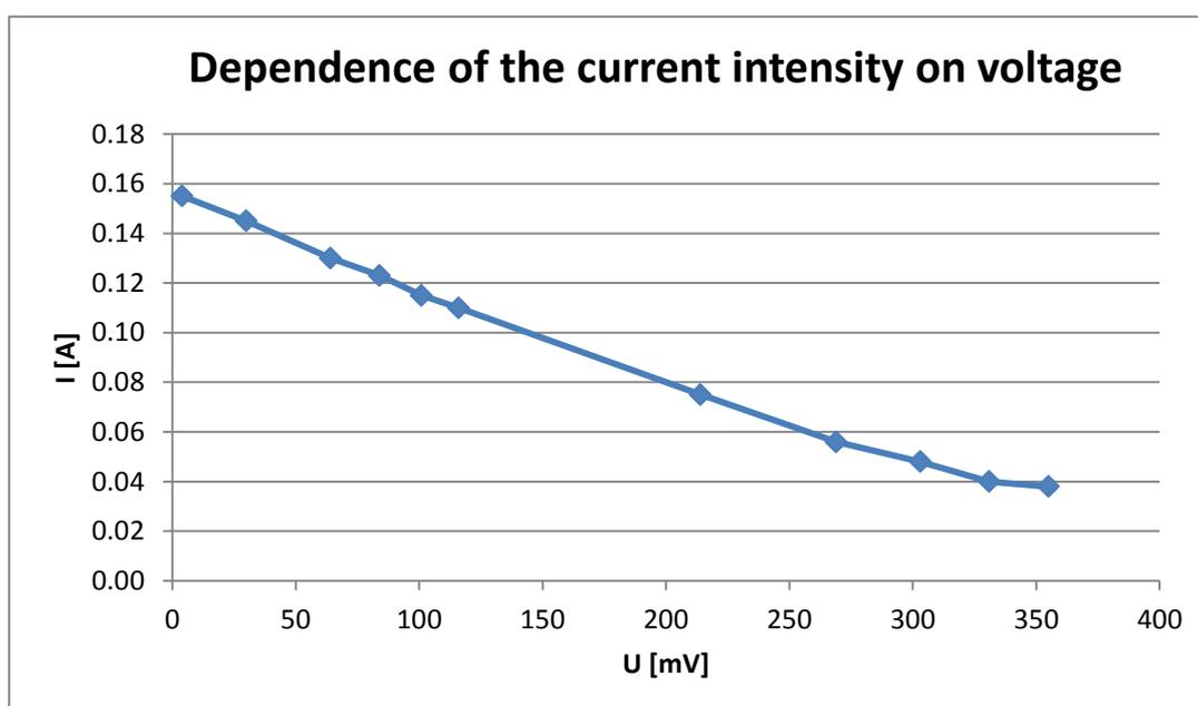
Figure 15. An example of the dependence of the current intensity on voltage for the working blueberry cell.
