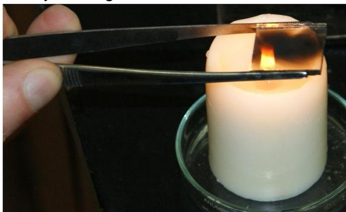
Figure 9. Covering the plate with the soot layer.
