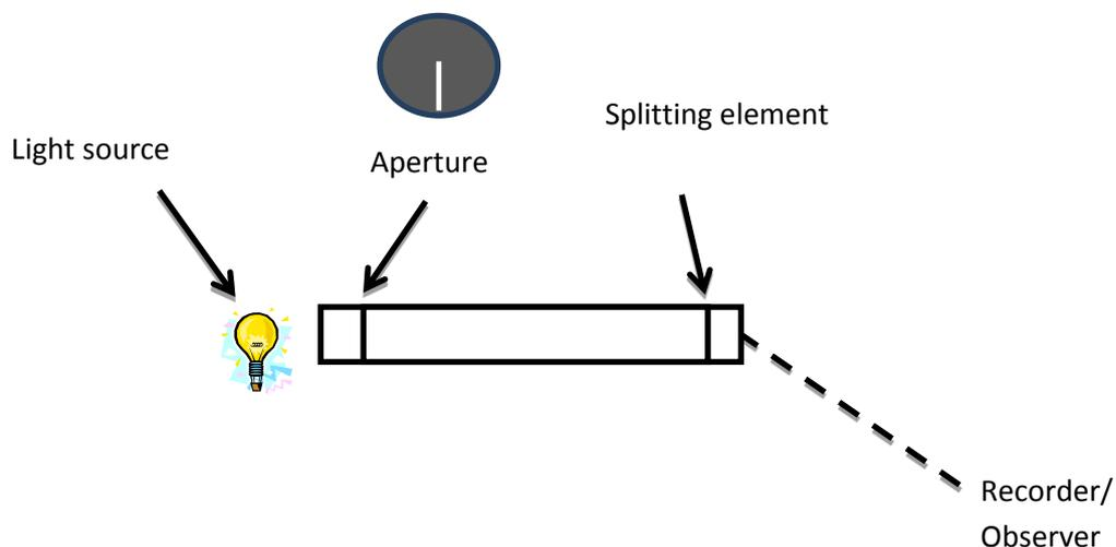
Figure 5: Diagram of a spectroscope
