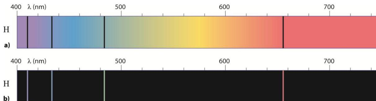
Figure 1. Hydrogen spectrum a) absorption spectrum, b) emission spectrum. (Derived from: *Physics for Scientists and Engineers (6th ed.)* by Serway and Jewett, Thomson Brooks/Cole, 2004).
