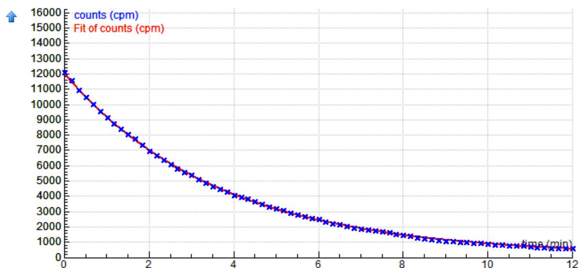
Exemplary data of the Barium-137m radioactive decay: measurement with MoLab data-logger and ML26m Radiation sensor, the coefficient of exponential function is  $\lambda = 0.272$ , the half-time  $t_{1/2} = \ln 2 / \lambda = 0.6931 / 0.272 = 2.548$  min.
