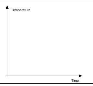
Now turn on the heater and record the inner temperature of the model house until it reaches a value of about +15  $^{\circ}$  C above the external temperature,  $T_{e}$ . Turn off the heater so that the temperature decreases until  $T_{e}$ .
