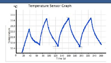
The graph above shows an experiment performed by a student that repeatedly switched on and off the heater, aiming at maintaining the temperature of the house at about 33 ° C. Try to calculate how much energy has been used if the heater was a 40W light bulb.
